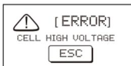
⇒ Voltage of one cell in the battery pack is too high.
