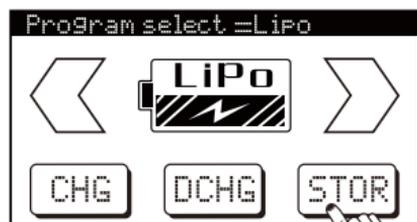
For different battery type, the end voltage are different, LiPo:3.85V, LiHV:3.85V, LiFe:3.3V, Lilon:3.75V. This is a intelligent program, it detects the battery voltage and automatically charge or discharge the battery. make sure to connect the battery to balance port when use this program.
