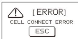
⇒ The battery balance connection is wrong. Please check the connector and cable.
