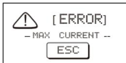
⇒ Output current is higher than setting in digital power mode
